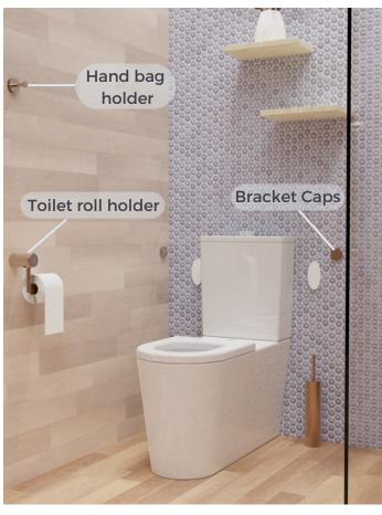
The toilet requires a grab rail on side and back walls and a backrest. The cistern can be in wall or standard, either option must have raised flush buttons. An extended toilet pan is also required.
