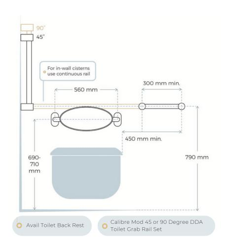
Both 45 and 90 degree rails are available. 45 degree is ideal however if space is limited the 90 degree is suitable.
