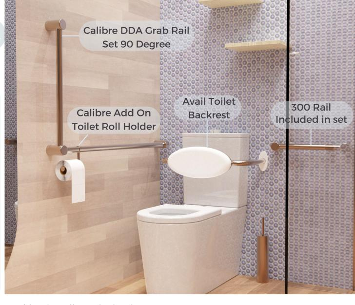
The toilet requires a grab rail on side and back walls and a backrest. The cistern can be in wall or standard, either option must have raised flush buttons. An extended toilet pan is also required.
